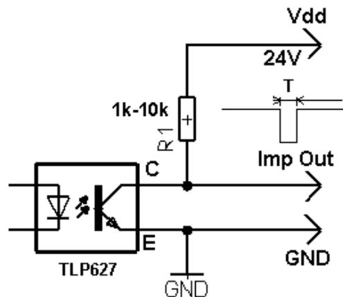
Owing to  $CTR \approx 100\%$ , it is necessary to select the collector current of 2.5mA at the most.
