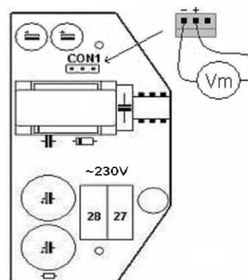
If the measured value is out of the given interval and the 230V mains is in order, the power supply unit is faulty. Its replacement without necessary recalibration is sufficient for the service.
