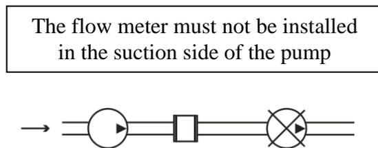
The flow of liquid in the flow sensor should be **steady and with no whirls**. For this reason, straight pipe sections of the same diameter as that of the sensor (permitted deviation +5%) are usually inserted before and behind the flow sensor. The minimum length of the sections is  $3 \times d$  before the flow sensor and  $2 \times d$  behind the flow sensor.
