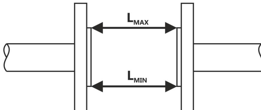
In the same way, the mating positions of holes for connecting bolts in counter-flanges should be ensured as well as ample room behind the flanges for the connecting bolts and nuts in order to ensure proper installation of the sensor in the pipe and the attachment by connecting bolts.
