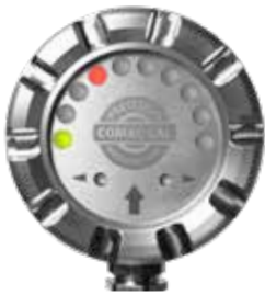
first LED flashing the flow below the monitor range
