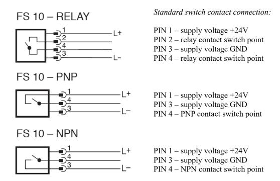
As a standard, the evaluation unit delivered for 24VDC±10%, 150mA power. The signal outputs of the monitor may be connected only to devices where the personal accident protection is ensured by a safe low voltage and where the generated voltages do not exceed limits specified for safe low voltage.
